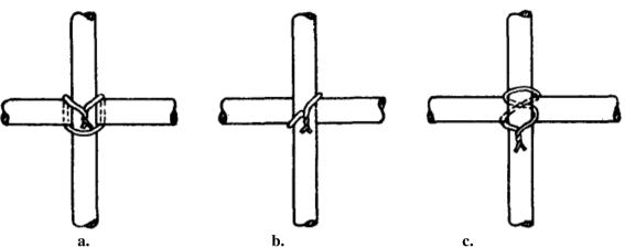
Figure 2.2 Three methods of trying reinforcement bars
