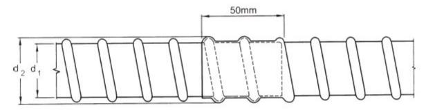
Figure 1.6 Typical details heat-shrink coupler
