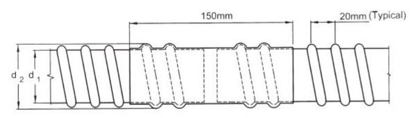
Figure 1.5 Typical details of a sleeve coupler
