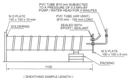
Figure 1.4 Test For Water Loss Study C1.7.2 Corrugated HDPE sheathing ducts
