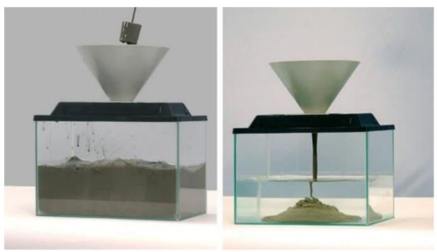
Figure 1.1 Without or With(right) Anti-washout Admixture
